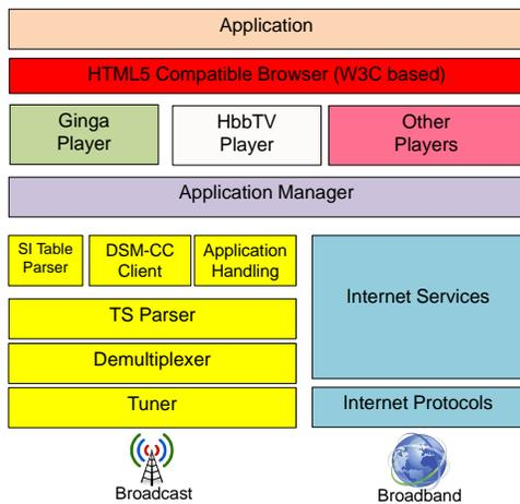
Fig. 3: Schematic block structure of a multi iTV system terminal for a coexistence approach
