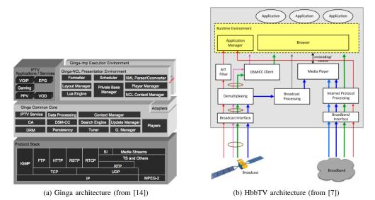
Fig. 2: iTV system architecture: Ginga (left) and HbbTV (right)
