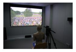
Fig. 6: Manikin for audio recording
