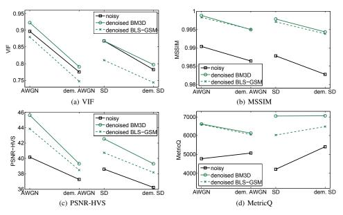
Figure 9. Quality metric results for the denoised test sequences using BM3D [4] and BLS-GSM [3].
