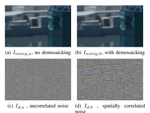
Figure 3. Crop of the sequence "City". Noisy image (left) and noisy image with demosaicking (right). In the second row the respective difference
