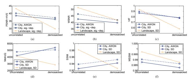
Figure 7. Quality metric results for the test sequences "City" and "Landscape" using the traditional AWGN model (dashed) and the realistic signal-dependent noise (solid lines). The uncorrelated noise, processed without demosaicking, is shown on the left, the results with demosaicking on the right.
