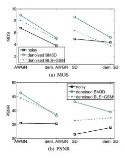
Figure 8. MOS and PSNR for the denoised test sequences using BM3D [4] and BLS-GSM [3]. The results using model (AWGN) are shown on the left, the results for realistic camera noise on the right.
