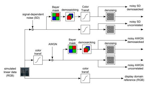
Figure 4. Processing of simulated sensor data for the test using signal-dependent noise (SD) and AWGN.
