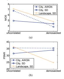
Figure 6. The MOS and PSNR results for the test sequences "City" and "Landscape" using the traditional AWGN model (dashed) and the realistic signal-dependent noise (solid lines). The uncorrelated noise, processed without demosaicking, is shown on the left, the results with demosaicking on the right.
